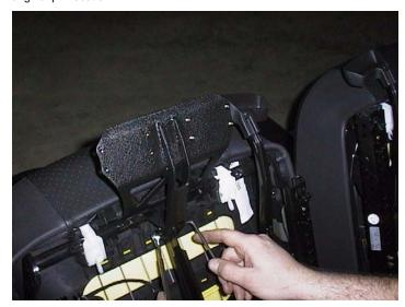
Step. 4 Install (2) screws and nuts through the existing holes on the seat bracket B as shown in figure 1 and fire Extinguisher mount.
