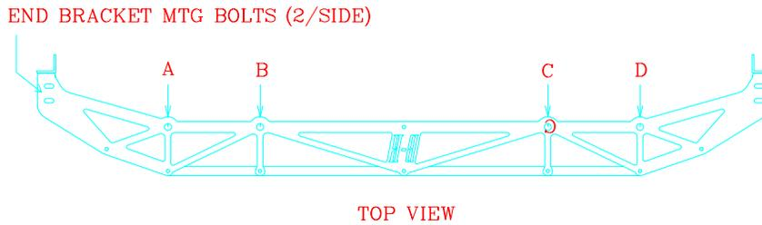
NOTE: Do not use bolt in plates other than 3/16" thick so that the overall height of the (2) spacers and plate are 1.00".
