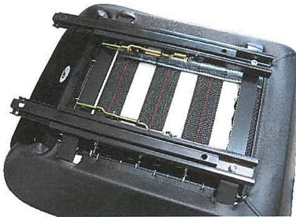
Attach the rail at the rear and hand tighten.
