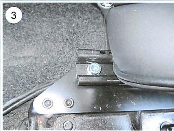
Attach the seats which have the rails already mounted to them. Using the handle, slide the seat all the way back exposing the front attachment holes of the rails. Using M8 x 25 bolts, flat washers and M8 Nyloc nuts, attach the rails to the brackets and tighten the nuts loosely.
