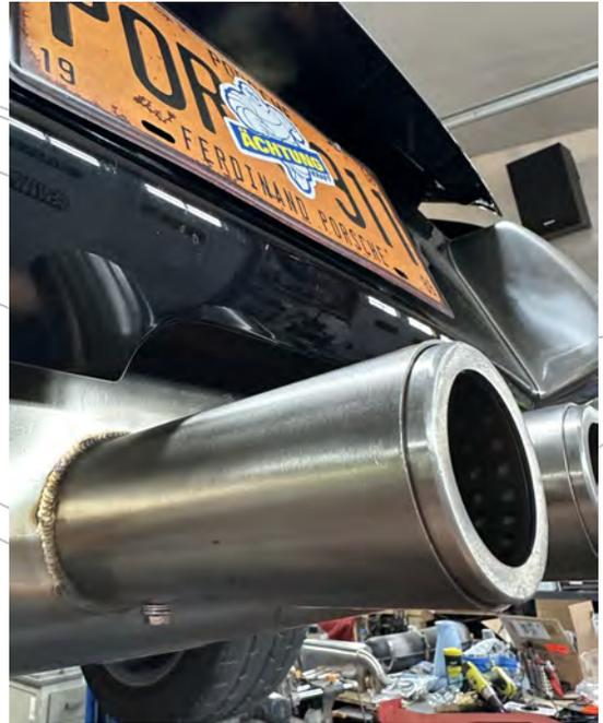
ALL GT/k mufflers come with silencer tips installed. For a louder and free-flowing OPEN/CLOSED experience, remove the lower bolt and slide the inserts out using the (included) hook awl and put the bolt in the silencer for storage.
