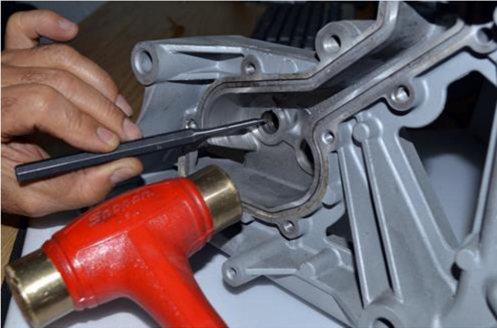
**Step 8:** Centre the punch and lightly hammer (tap) a small hole in the IMS cover. (1-3MM)
