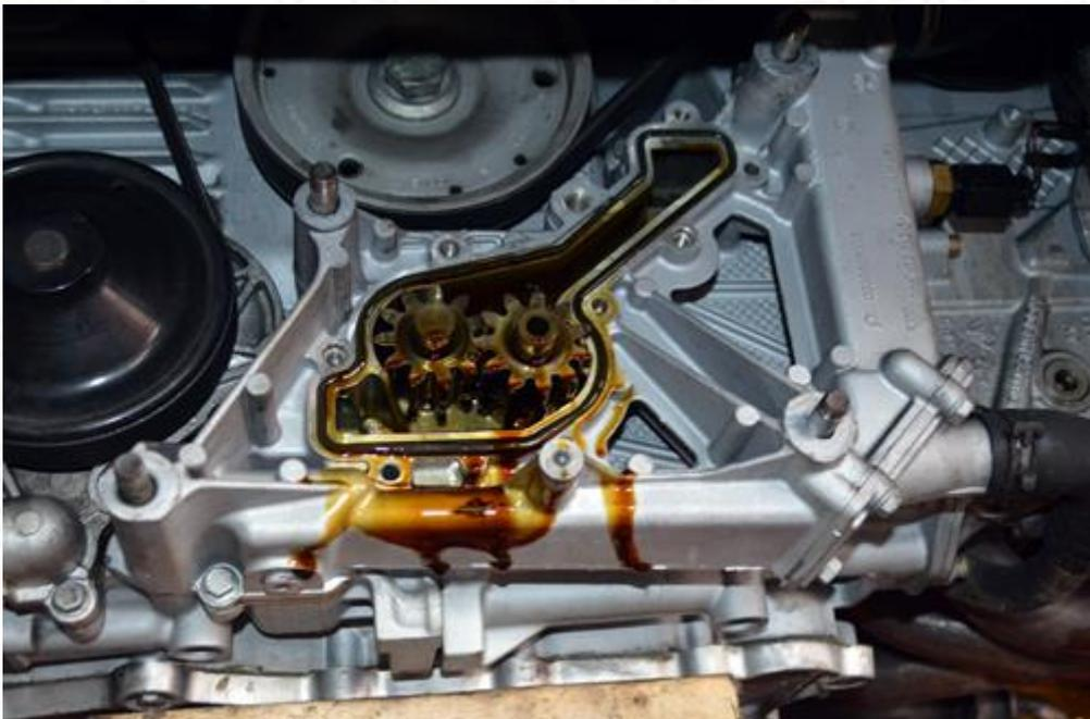
**Step 5:** Remove the Oil Pump Drive (8MM Allen)
