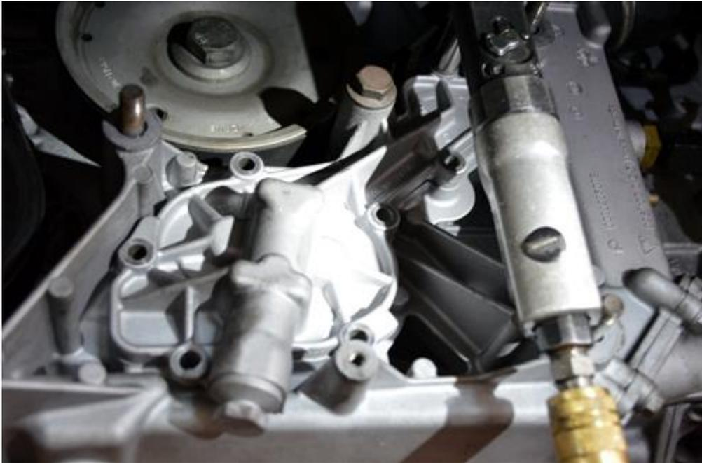
**Step 4:** Remove the Oil Pump Gears
