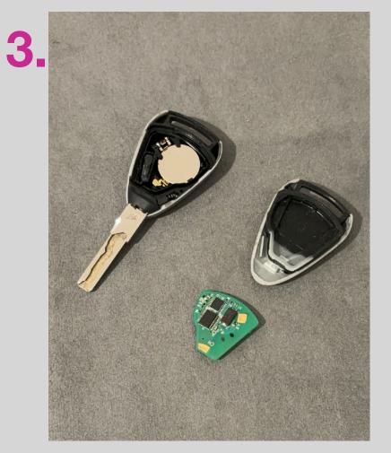
Opening the two sides, remove the PCB from the rubber cover.
