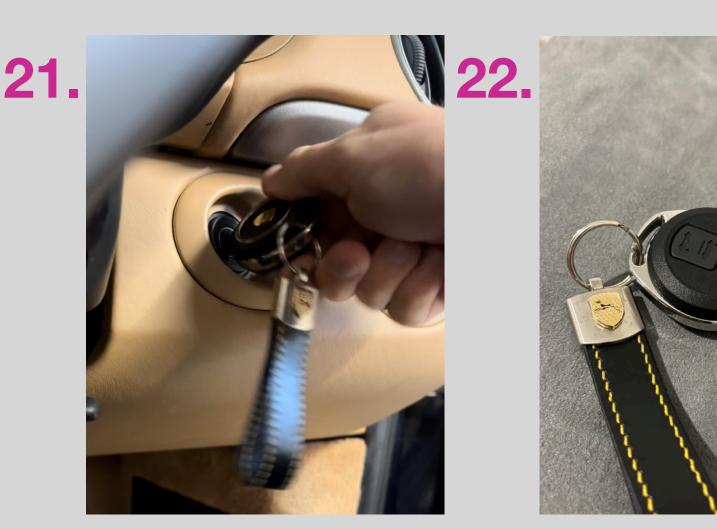
With any battery replacement - your key may need a reset. To do this, simply place the key into the ignition and turn to engage the ignition (not starting the car). Press and hold the lock button for 15 seconds. The horn may sound when this step is complete.
