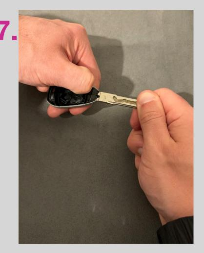
Pull back the slider and remove the key blade.
