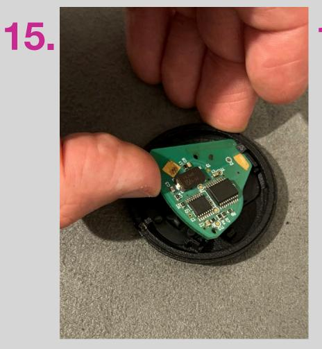
Place the pointed end into the side with a single hook. Pushing the rear in last.
