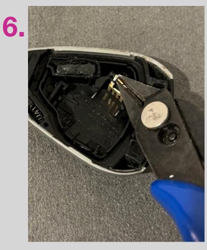
Using tweezers or grips, carefully remove both of the brass connectors. Be sure to hold the connectors where there is more material to avoid damage.
