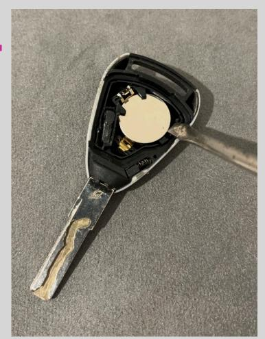
Remove the coin battery from the casing.
