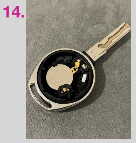
Carefully press the brass contactors into place, using the screw driver to gently push them firmly into the fittings. The coin battery can then go in. Add the transponder pill back to the casing. Angled face pointed forward and down (towards the badge).
