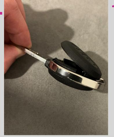
Using the slot on the button side of case, place the back end down first.
