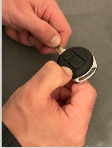
In a circular motion, press around the key casing so that the case is properly sealed.
