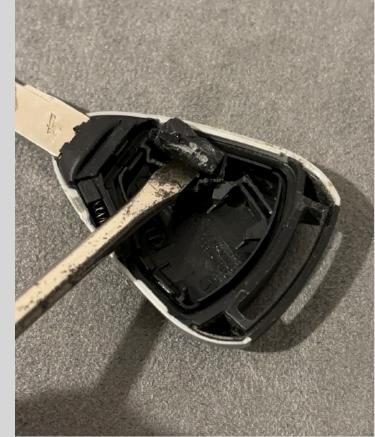
Using the screw driver you can pry the transponder pill out of the casing. Note which way the pill points.
