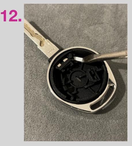
Insert the key blade and push the pin into the forward position to lock the key in place.
