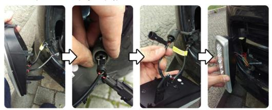
4. Find the ACC/Ignition power in engine room, connect the red wire to ACC. Route the main harness properly in the engine room, and connect to the driver side and passenger side LED DRL lights (harness to LED DRL light is plug and play).
