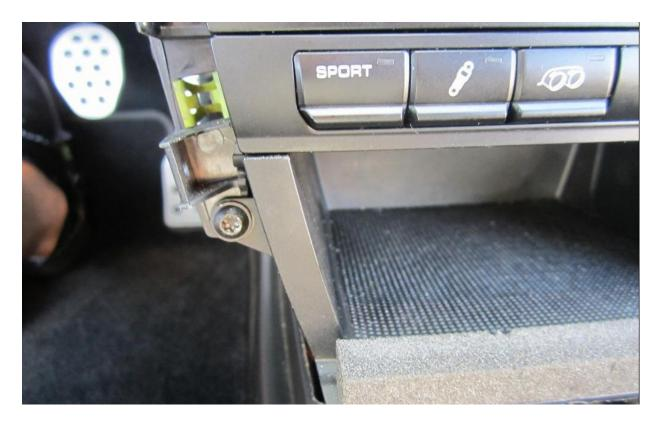
**8.** You are ready to pull the console out but first locate the wire connector on the inside right front of the console and disconnect it. Have the emergency brake handle pulled up. Pull the console up and out of position.
